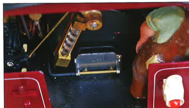
Above: A view into the smokebox showing the two flue tubes and the position of the exhaust and blower.
