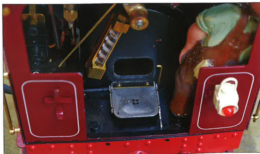
Above right, right and below: Three views of the fire door showing it shut, open with the damper and fully open for feeding.
